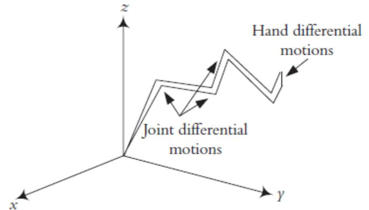
**(b) differential motions of the robot joints and the endplate**
