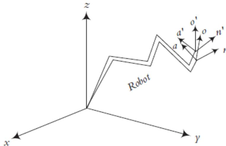
**(c) differential motions of a frame caused by the differential motions of a robot**
